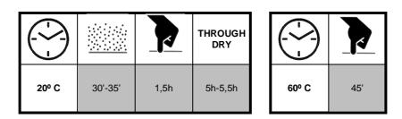
Maximum physical-chemical resistance is obtained after drying at room temperature for 15 days or 7 days when oven dried.
